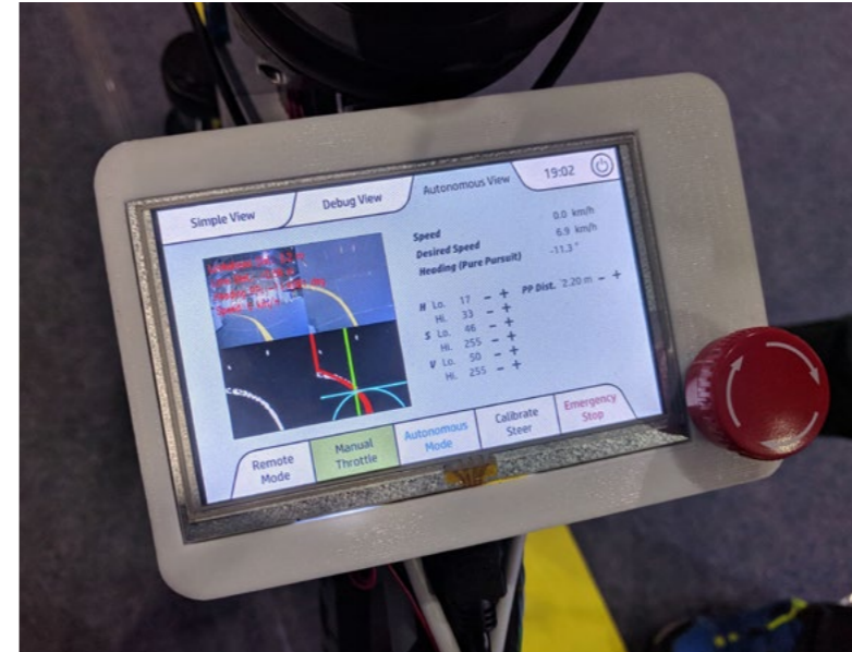
▲ Digital Instrument Cluster and its UI using Qt and QML (Apr 2019)
