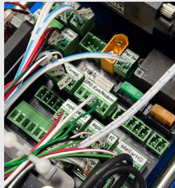
▲ Internal Wiring Configuration of the PKRC Underwater Robot (May 2025) Interne Verkabelung des PKRC-Unterwasserroboters (Mai 2025)
